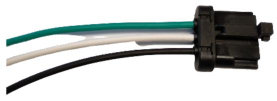
7. Slide the red lock tab into the front of the connector as shown. Then press it in until it is flush and snaps into place (this will require some force).
