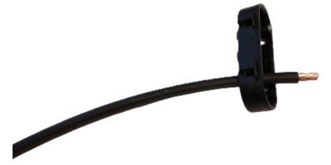
3. Slide the blue rubber seal over the wire as shown.
